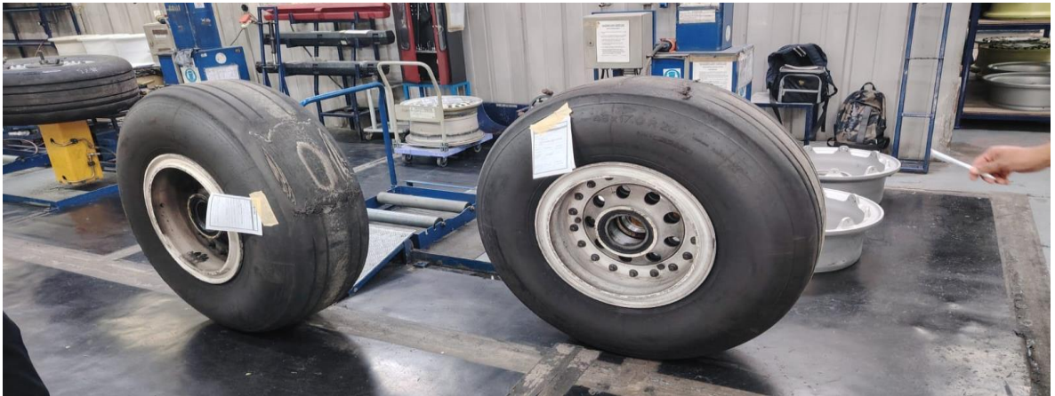
Figure 2: Showing damages sustained on the right main tires (number 1 and 2).
