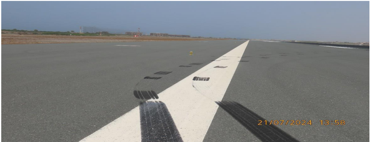
Figure 7: showing evidence of left wheel tire marks showing anti skids jerking outside the left edge of the RWY 08L while turning right into the RWY 08L, towards Taxiway Y6.
