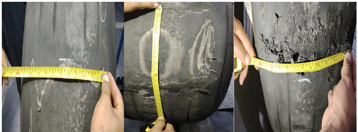
Figure 8: showing evidence close view of the main wheel tire damages.
