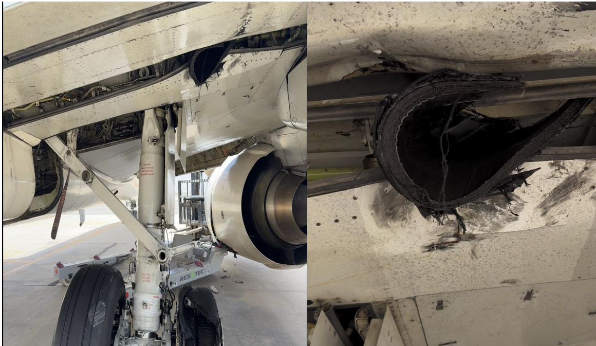
Figure 7: Shows the hydraulic leak due to tire burst and flap damage.
