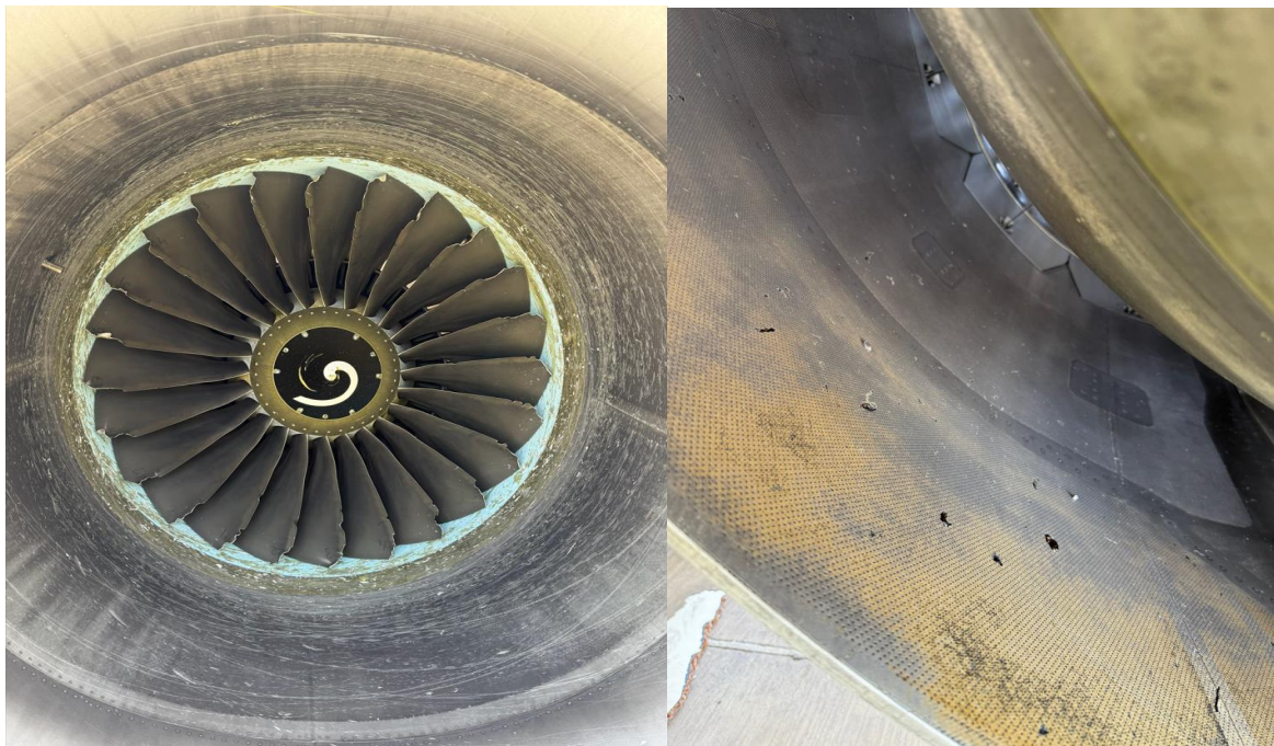
Figure 8: Shows the damage in engine No.2.
